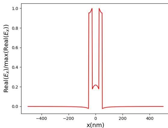
Figure 5: The distribution of the normalized  $E_x$  component along the  $x$ -axis and the middle of the waveguide.
