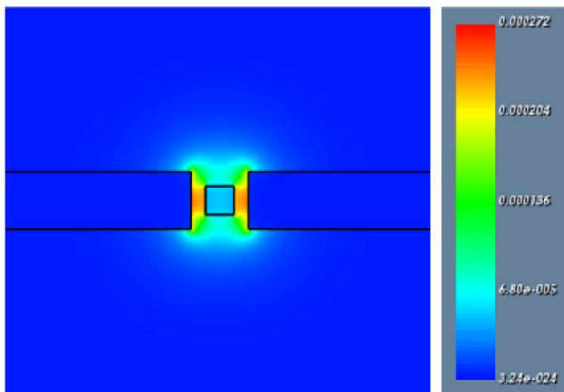
Figure 4: The Poynting vector distribution in the  $z$ -direction for a waveguide with geometrical dimensions  $W = 100 \text{ nm}$ ,  $H = 100 \text{ nm}$ ,  $w = 50 \text{ nm}$ , and  $h = 50 \text{ nm}$ .
