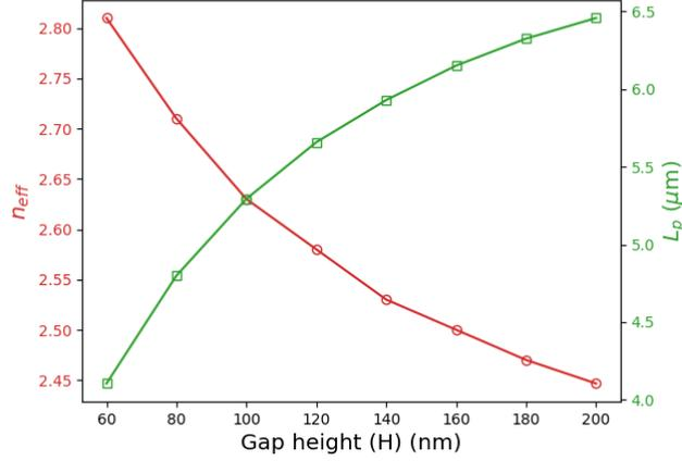
Figure 3: The effective index and the propagation length for a PFSPWG with different gap height and fixed core dimensions ( $w = 50 \text{ nm}$ , and  $h = 50 \text{ nm}$ ).
