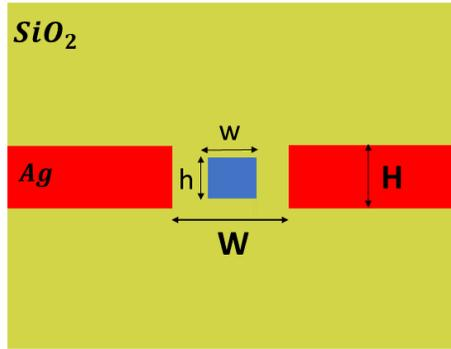
Figure 1: Schematic showing the cross-sectional view of the partially-filled slot plasmonic waveguide.
