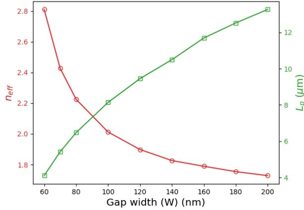
Figure 2: The effective index and the propagation length for a PFSPWG with different gap width and fixed core dimensions ( $w = 50 nm$ , and  $h = 50 nm$ ).
